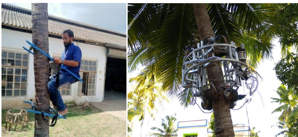
Fig.1 TNAU coconut climber and Amaron Robotic coconut climber
