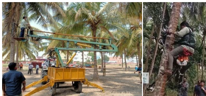
Fig.2 TNAU Coconut hoist and Climbing bike
