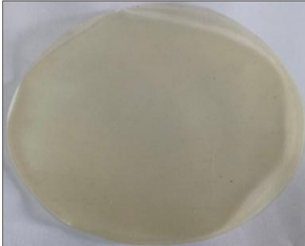
Fig. 1: Optimized film consists of CornStarch, Whey protein Concentrate, Whey protein Isolate, Polyvinyl Alcohol, Carrageenan and Glycerol
