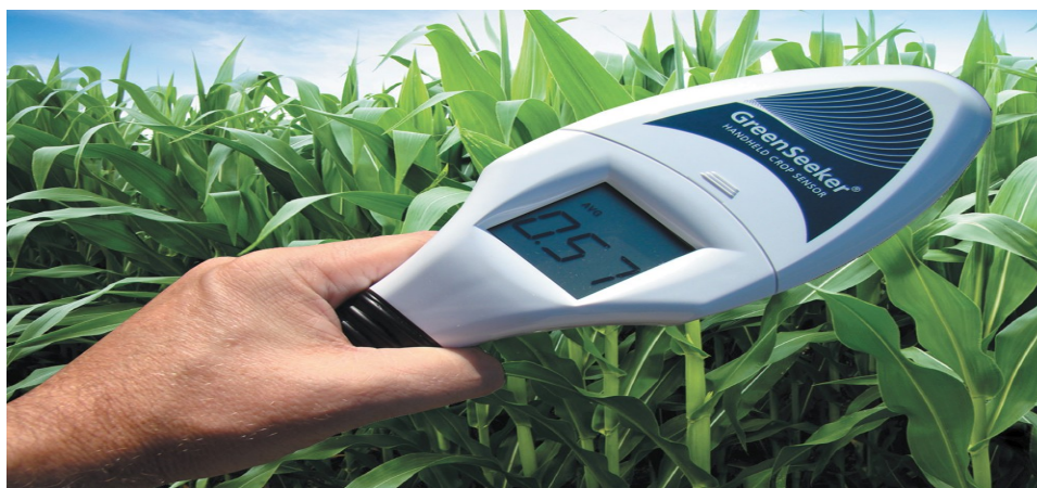
Fig. 3: Use of green seeker under field conditions
